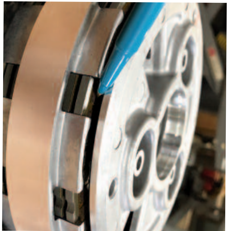
Photo #2. Not seated - see gap. Clutch will not work. Install friction steel friction on the pressure plate and hold as one unit while sliding on to locate teeth on the inner hub. They must mesh and sit flat like in Photo #1.
